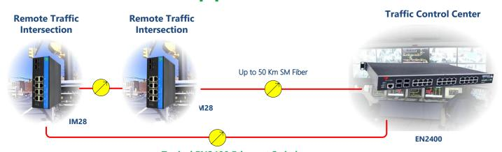
Typical EN2400 Ethernet Switch In Traffic Monitoring Redundant Configuration
