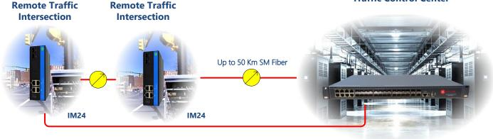
Typical IM24 Ethernet Switch In Traffic Monitoring Redundant Configuration
